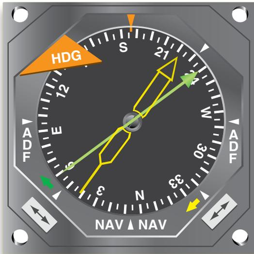
Figure 16-31. Radio magnetic indicator.
